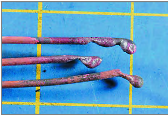
Figure 6.6.2.1(d) Copper Conductors Heated by Fire and Exhibiting an Extended Area of Damage. This damage was created during a test burn.
