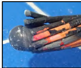
Figure 9.10.3.1 Rounded globule of formerly molten oxide formed after the molten oxide on a stranded conductor severed while carrying the load current.
