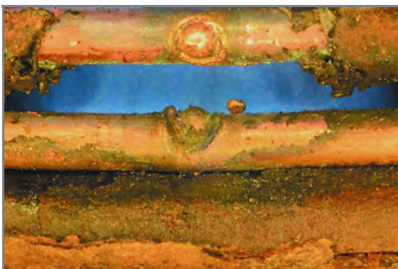
Figure 6.6.5.3.2(k) A Bead Within a Notch Created by an Electrical Arc on a Nonmetallic Sheathed (Type NM) Cable. The ungrounded (i.e., hot) conductor is at the top of the image. This damage was created during a lab test.
