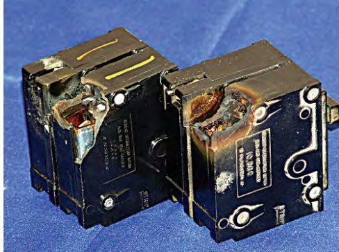
Figure 9.10.3.2(c) Overheated Connection on 240 V Dryer Outlet.
