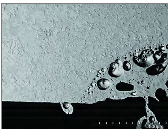
Figure 6.6.5.3.2(n) Locally Enlarged Grain Size of the Resolidified Material of an Arc Site after Cross-Sectioning. This damage was created during a lab test.
