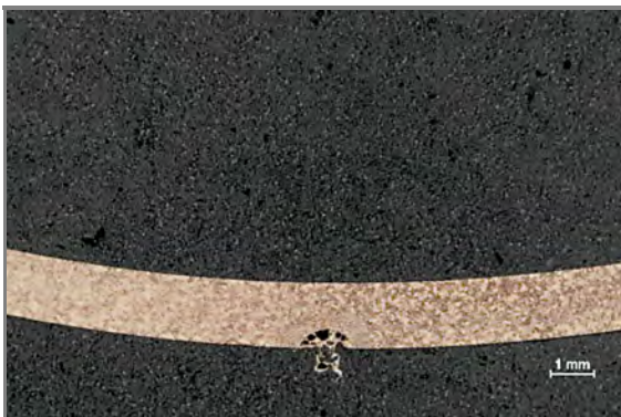
Figure 6.6.5.3.2(m) Close-Up View of Figure 6.3.21.5.3(l) with High Internal Porosity.
