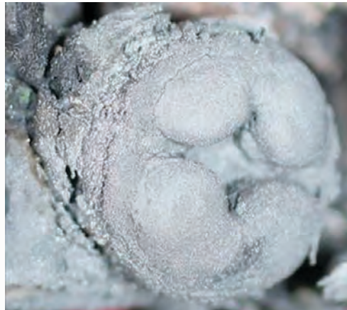
Figure 9.10.3.3(c) Enlarged Screw Head on Duplex Outlet Resulting from Severe High-Temperature Oxidation Corrosion and Adjacent to Glowing Connection.
