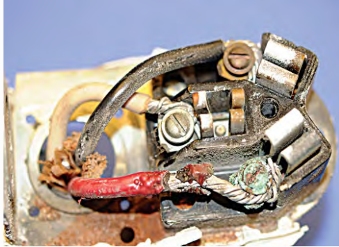
Figure 9.10.3.2(d) Overheated Connection on 120 V Duplex Outlet.
