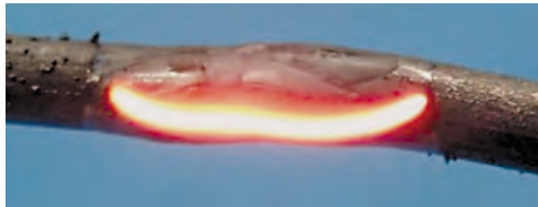
Figure 9.10.3 Filament of Liquid Oxide Present During the Overheating Process After Two Solid Wires Were Severed and Then Brought Back into Contact While Carrying Electrical Current.
