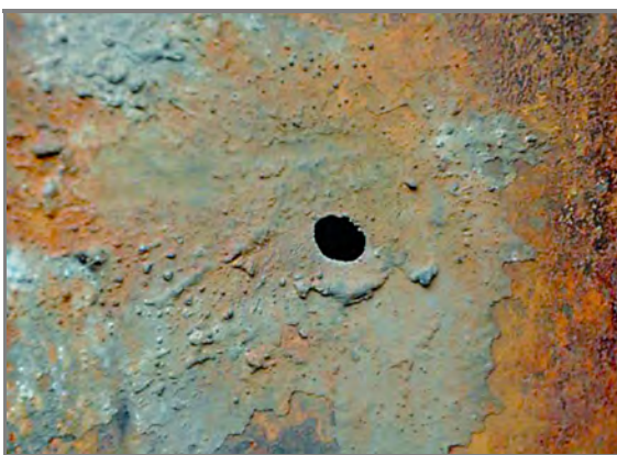
Figure 6.6.5.3.2(f) An Arc Site on a Nonmetallic Sheathed (Type NM) Cable that Exhibits Resolidification Waves. The ungrounded (i.e., hot) conductor is at the top of the image. This damage was created during a lab test.
