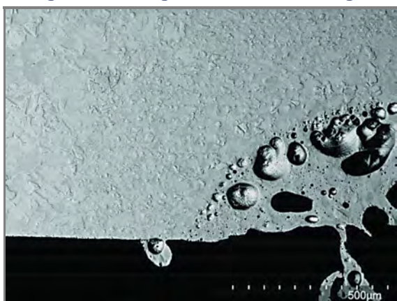
Figure 6.6.5.3.2(n) Locally Enlarged Grain Size of the Resolidified Material of an Arc Site after Cross-Sectioning. This damage was created during a lab test.
