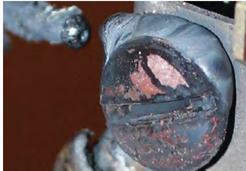
Figure 9.10.3.3(c) Enlarged Screw Head on Duplex Outlet Resulting from Severe High-Temperature Oxidation Corrosion and Adjacent to Glowing Connection.
