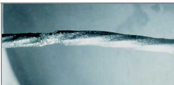
Figure 6.6.2.1(h) Copper Conductors Heated by Fire and Exhibiting Round or Irregular-Shaped Globules. This damage was created during a test burn.
