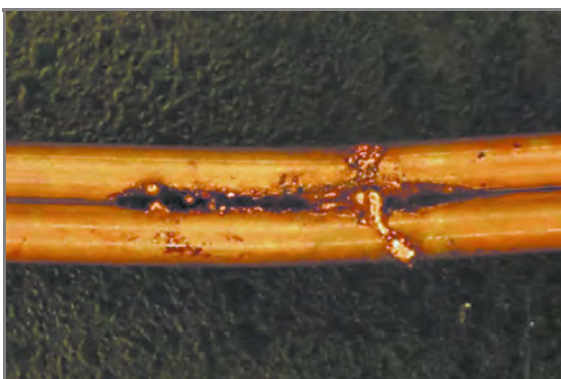
Figure 6.6.5.3.2(j) Nonmetallic Sheathed (Type NM) Cable with Rounded or Irregular-Shaped Beading Created by an Electrical Arc. The ungrounded (i.e., hot) conductor is at the top of the image. This damage was created during a lab test.
