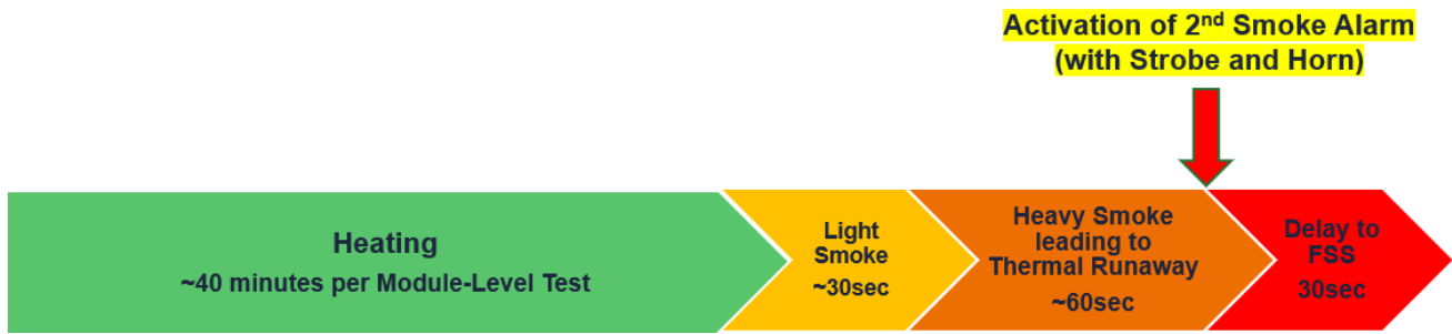
Figure 25 Stat-X Fire Suppression System Activation Sequence
