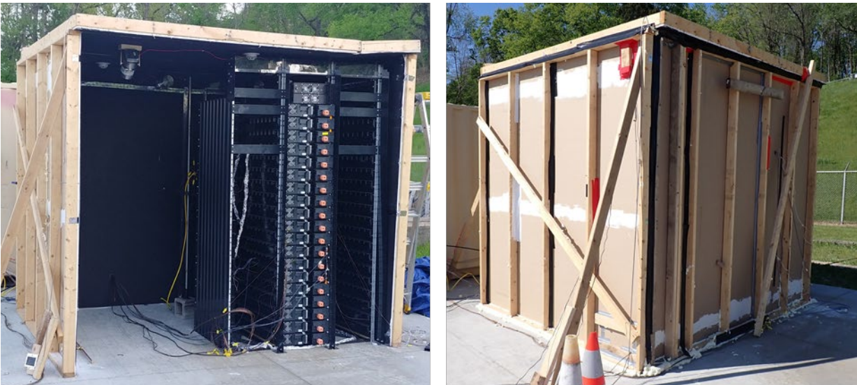
Figure 13 Mock-up test enclosure with the front wall in place (right) and without the front wall in place (left)
