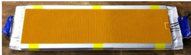
Figure 4 JH4 Cell with Installed Flexible Film Heater
