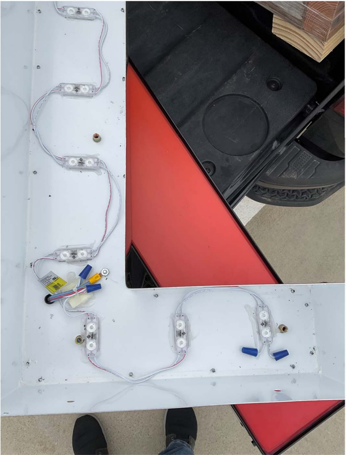
Remote wired Class 2 channel letter metal bonded. 3 wire Class 2 cable installed.
