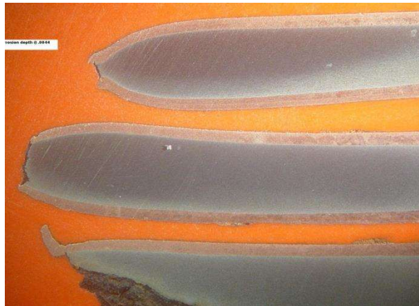
Figure 4a: There is no visible corrosion between the copper and steel on all wires obtained from the substation in Kentucky.
