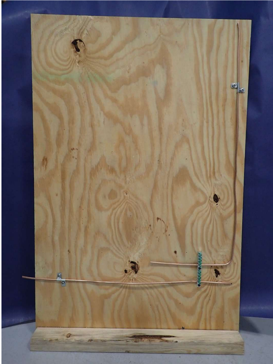
Figure 6. Example busbar and 4 AWG GEC test setup.
