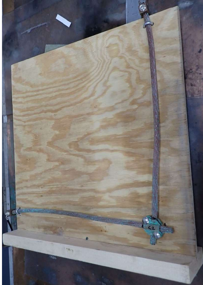
Figure 11. Example cross connector assembly following the corrosion conditioning process.
