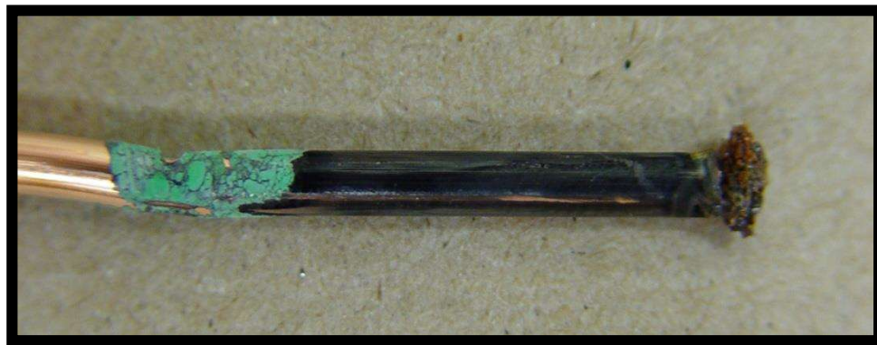
Figure 1: Example of Underground Corrosion of Copper Clad Steel
