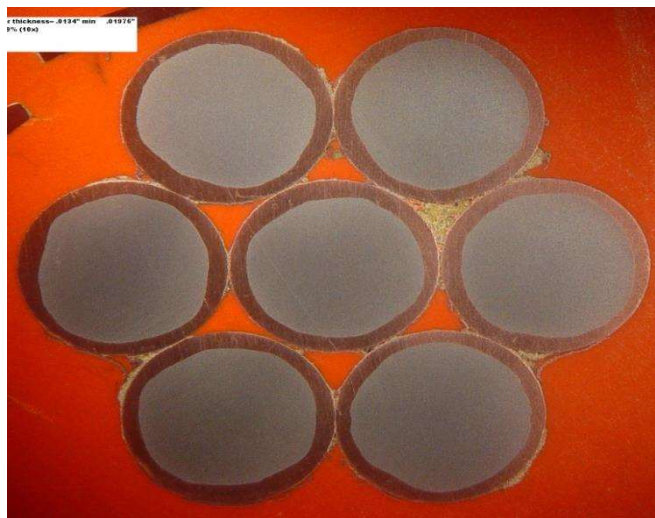
Figure 3: Copperweld® 40% LC DSA 7 No. 5 manufactured in 1962
