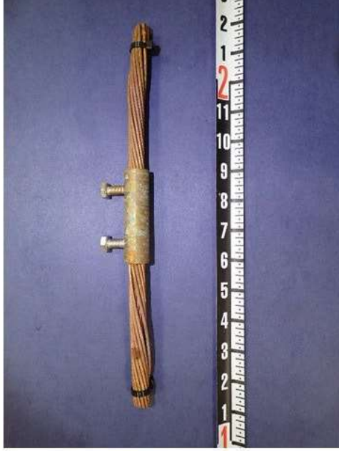
Figure 4. Representative photographs showing the straight connector samples before and after testing for Cu (top row) and CCS (bottom row). The zip ties were removed for testing.
