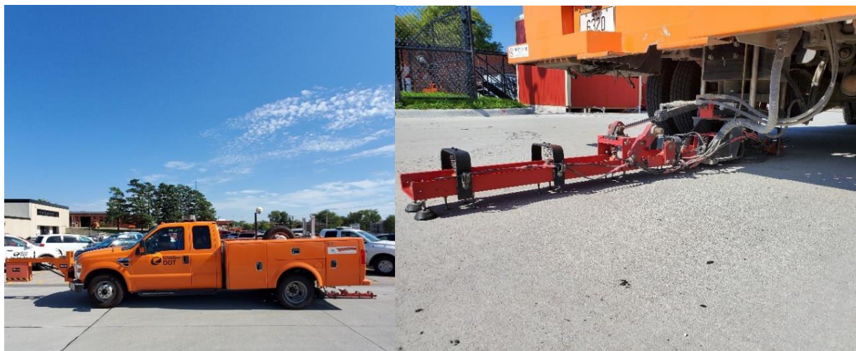
Figure 46. Iowa DOT FWD vehicle
