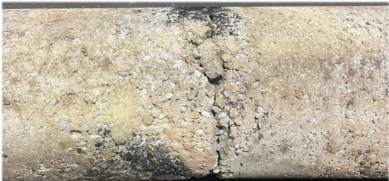
Figure 12 - Carbonate concrete block appearance after the test
