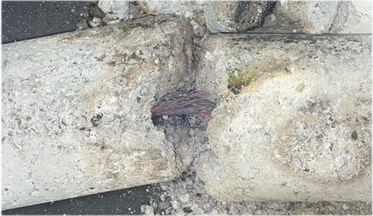
Figure 13 - Carbonate concrete block opened after the test showing heat damage to the insulation
