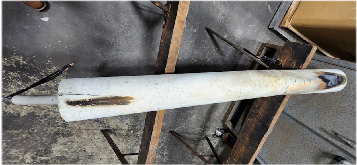
Figure 9 - Siliceous concrete block appearance after the test
