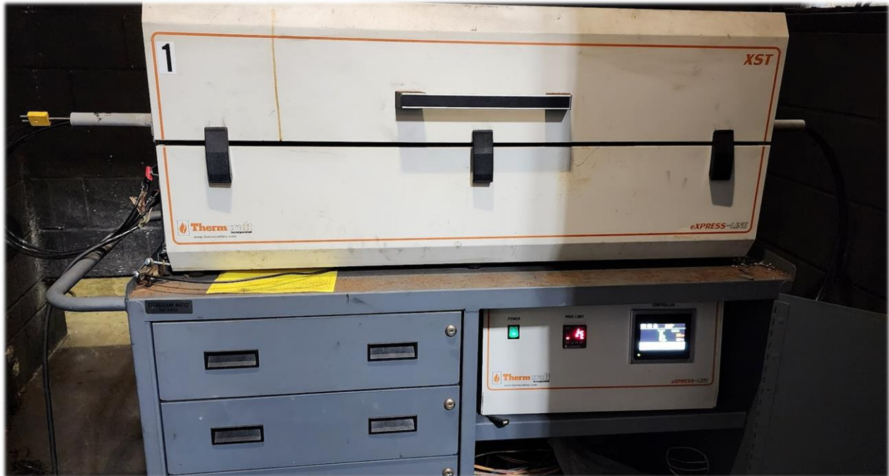
Figure 5 - Tube furnace containing the concrete block and wires
