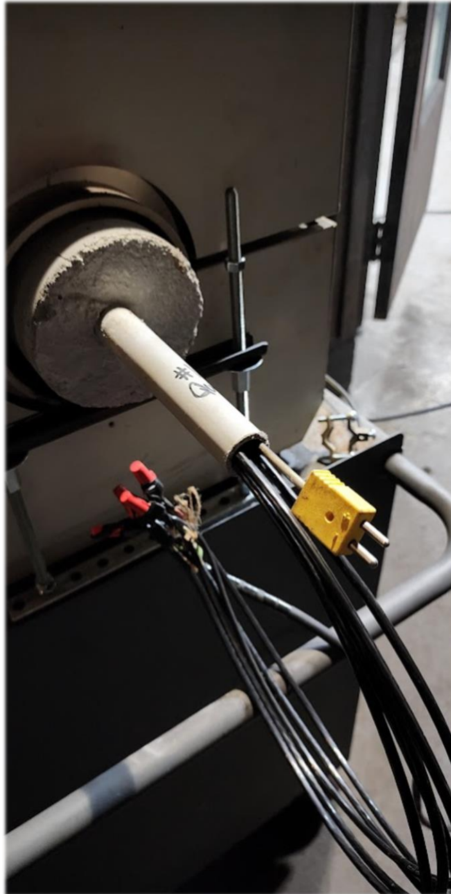
Figure 4 - Thermocouple and wires inside conduit and inside tube furnace
