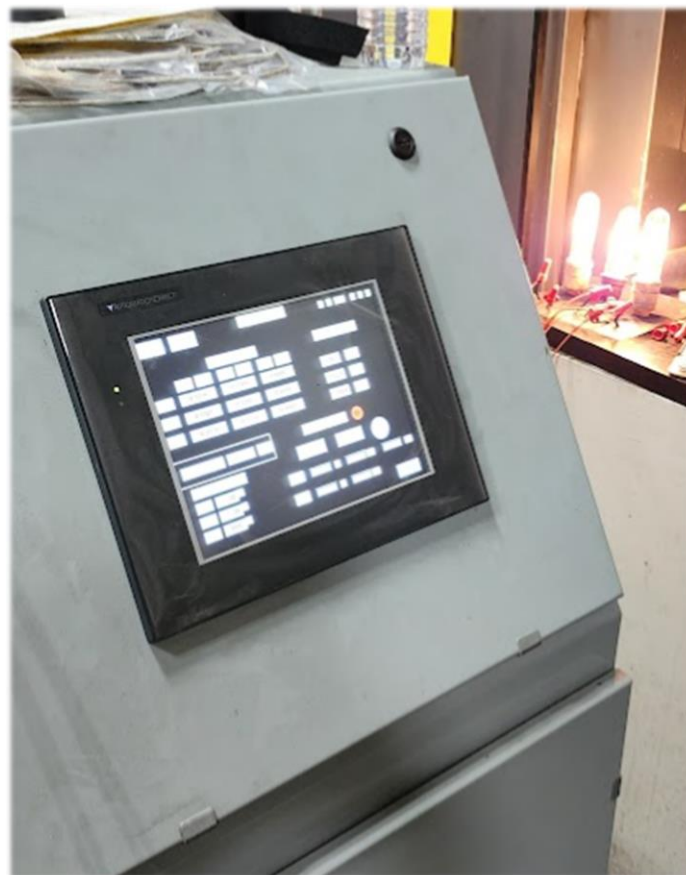
Figure 6 - Data acquisition device connected to light bulbs as the load
