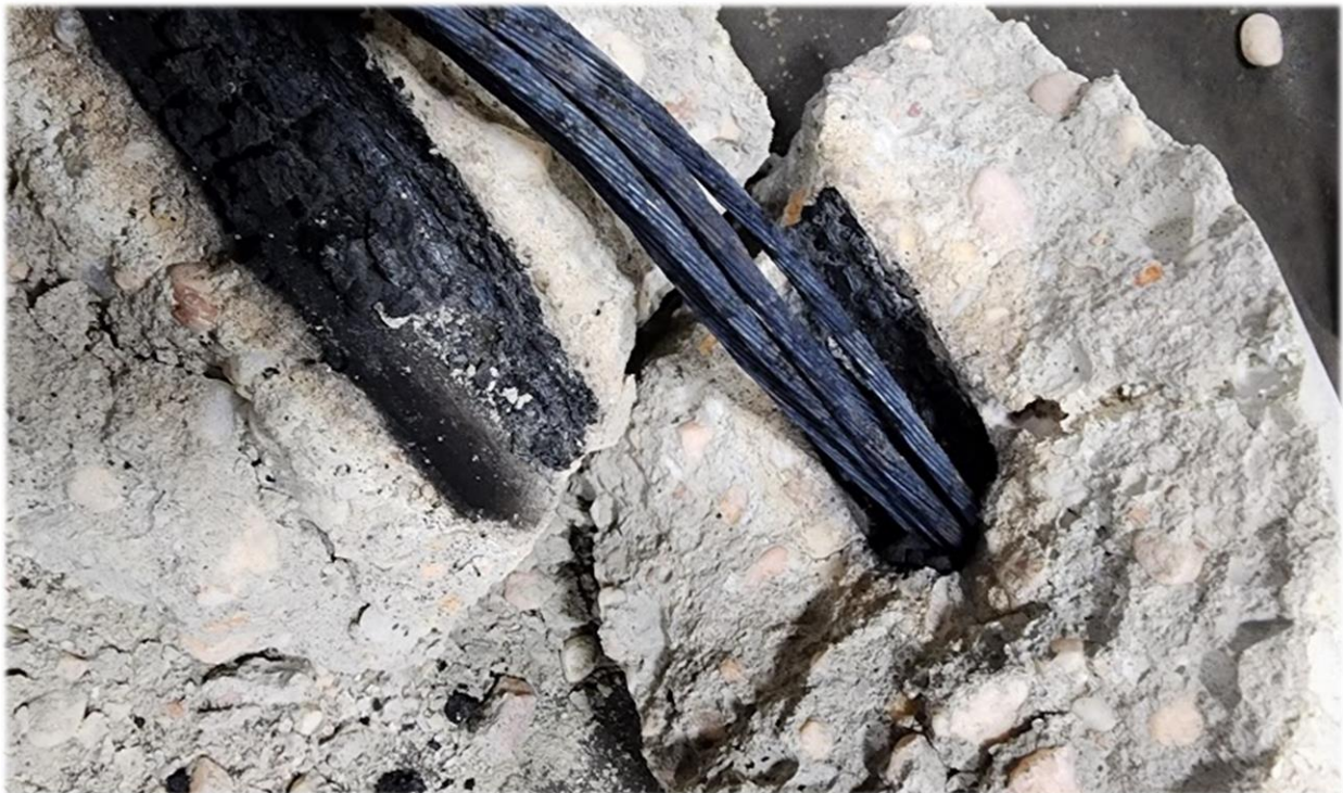
Figure 10 – Siliceous concrete block opened after the test showing heat damage to the insulation
