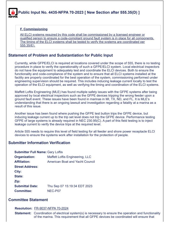
devices upstream of a fault continue to operate, so as to not interrupt power of the entire marina electrical system.
