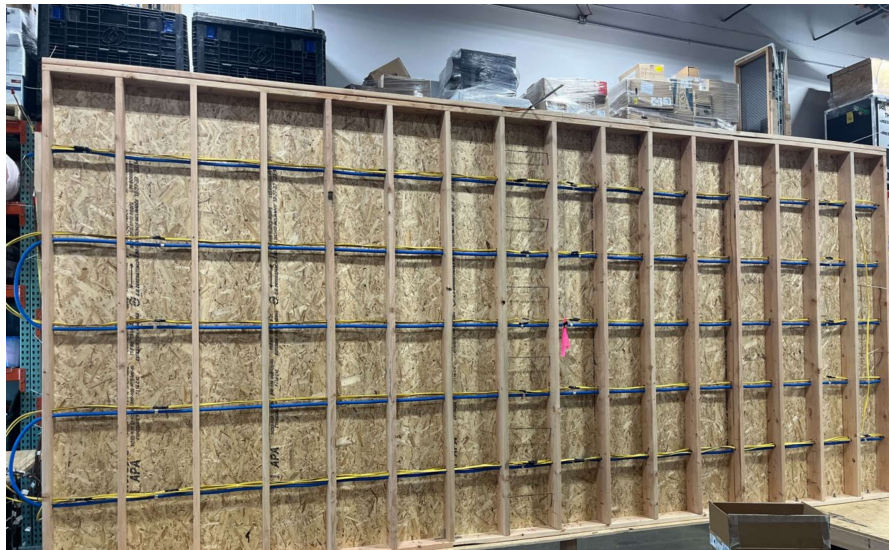
Figure 1. Test fixture, seen without fiberglass blown-in insulation and foam board insulators, used in Copperweld's July 2024 tests.
