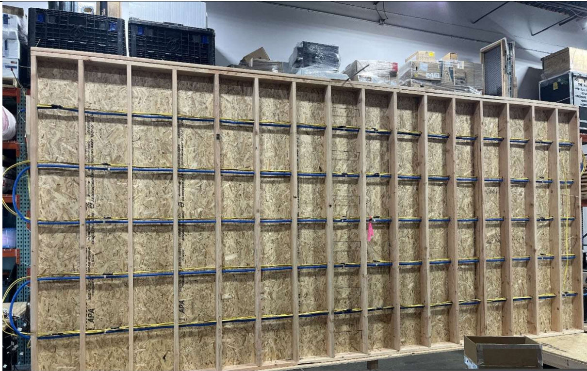
Figure 10 – Thermocouple Location on NM-B Cables
