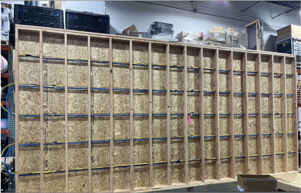
Figure 4 – Test Fixture with Conductors Installed
