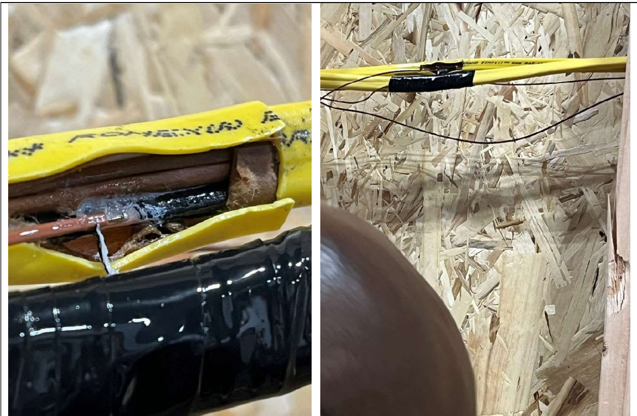
Figure 11 – Thermocouple Attachment to Bare Conductor and Jacket Closed
