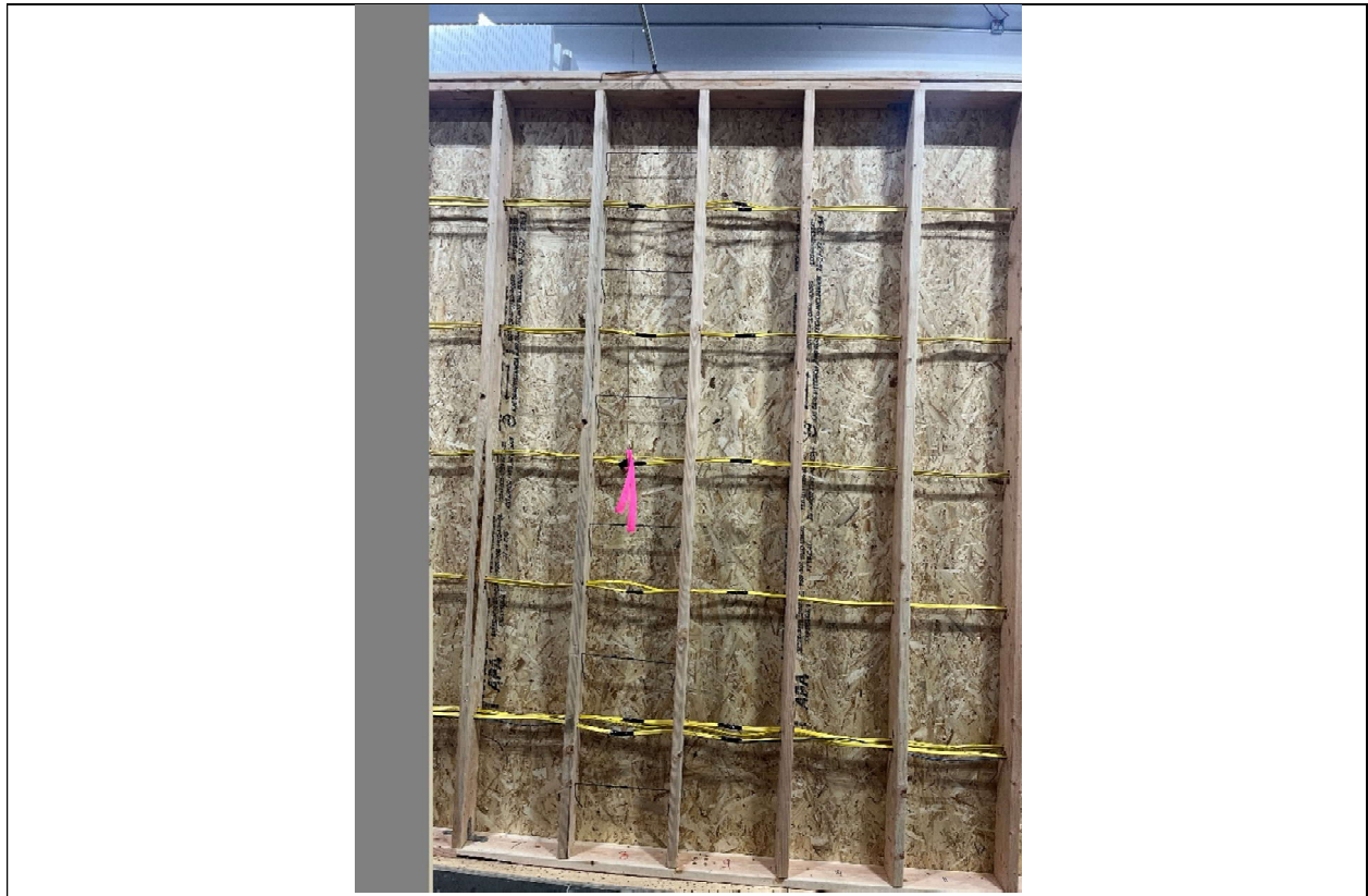
Figure 7 – Inter Level Thermocouples Between Conductor Levels on Paracord
