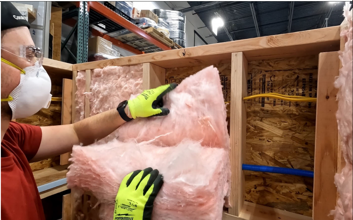
Photo 6 – Test Fixture 1 R-21 Fiberglass Insulation
