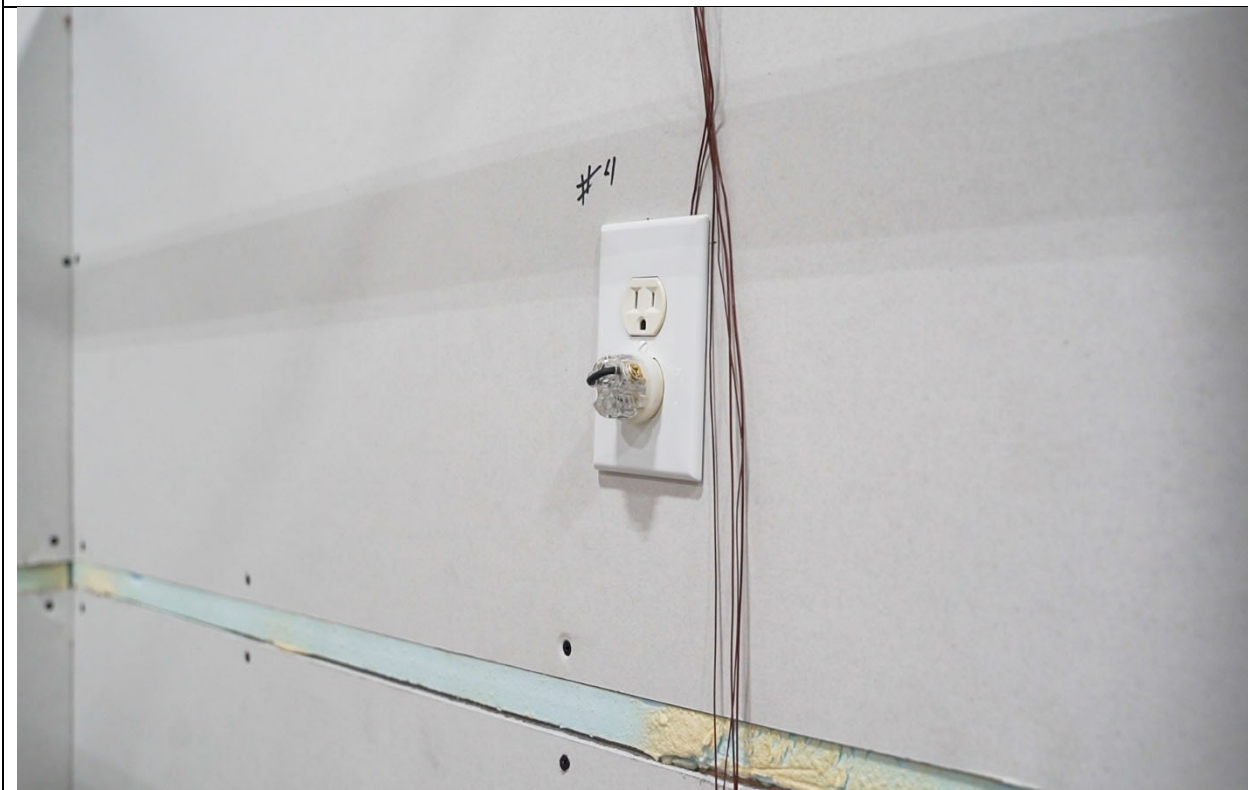
Photo 12 – Receptacle with Thermocouple and Shorting Plug
