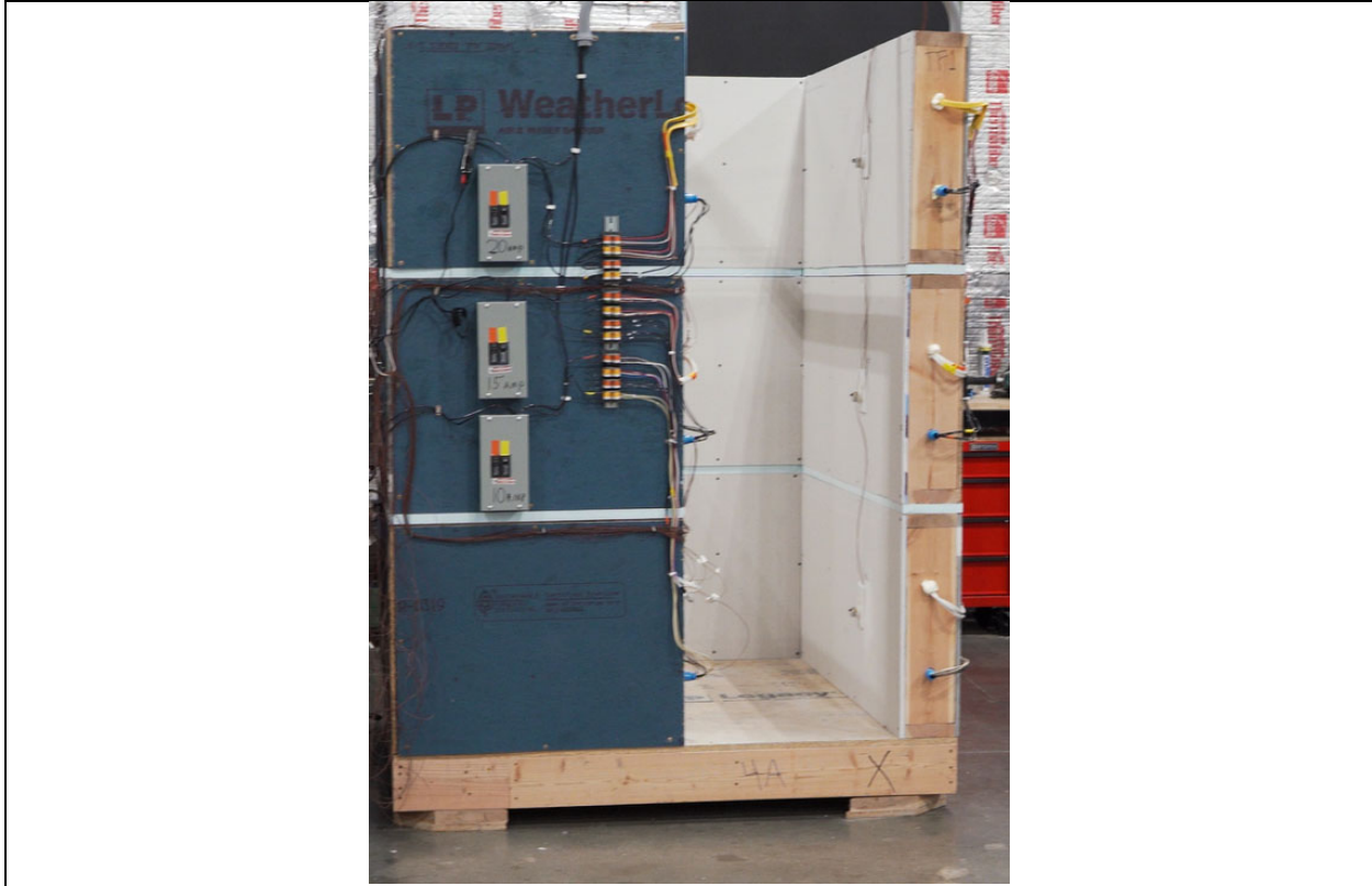
Photo 11 – Wall Fixtures Supply Circuit Breakers
