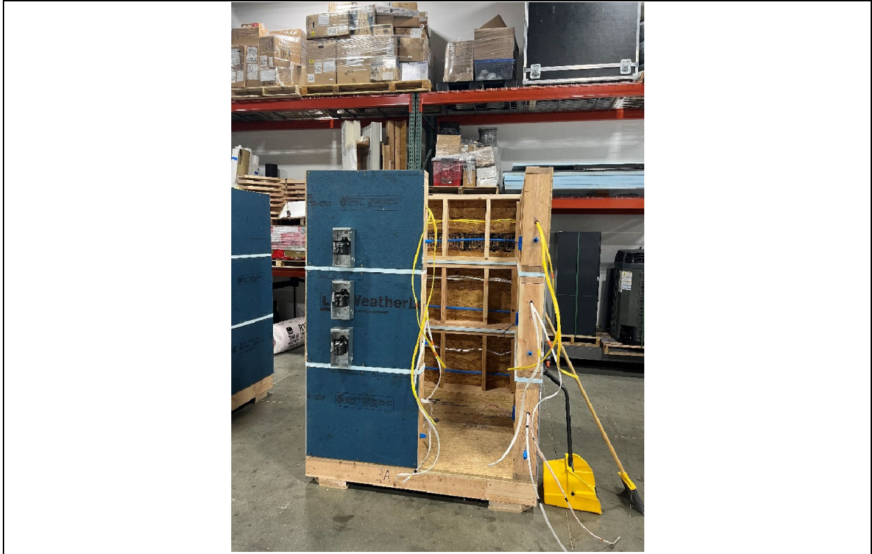
Photo 3 – Wall Test Fixture with Rough Wiring Installed
