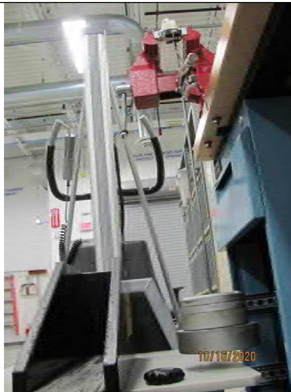
Photo 10 – Pull Out Test Suspended Weight
