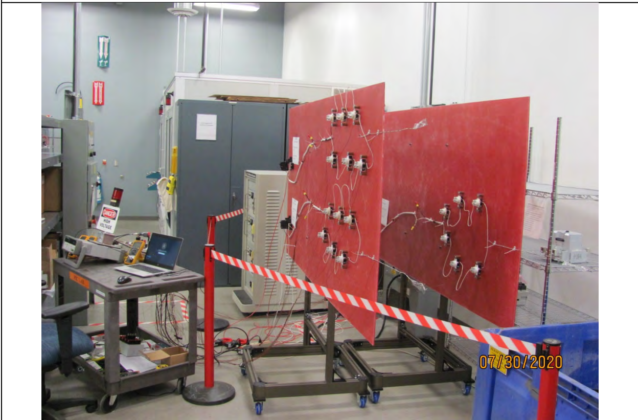
Photo 2 – Test Board and Test Equipment Arrangement
