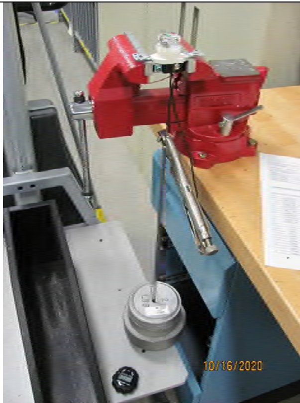
Photo 9 – Pull Out Test Setup
