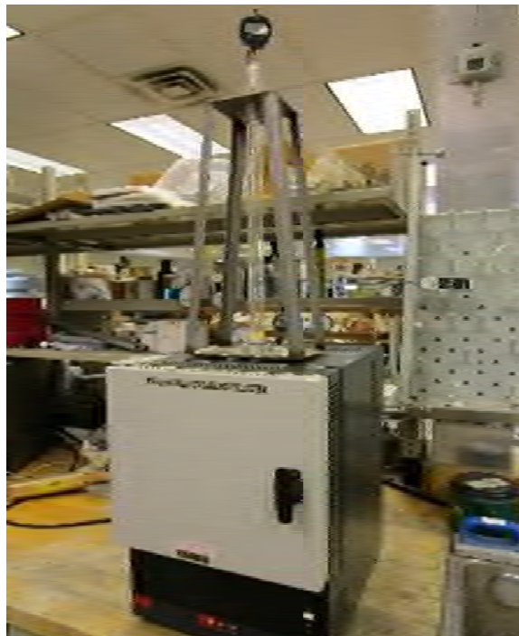
Photo No. 2 ASTM E228 - Equipment Detail
