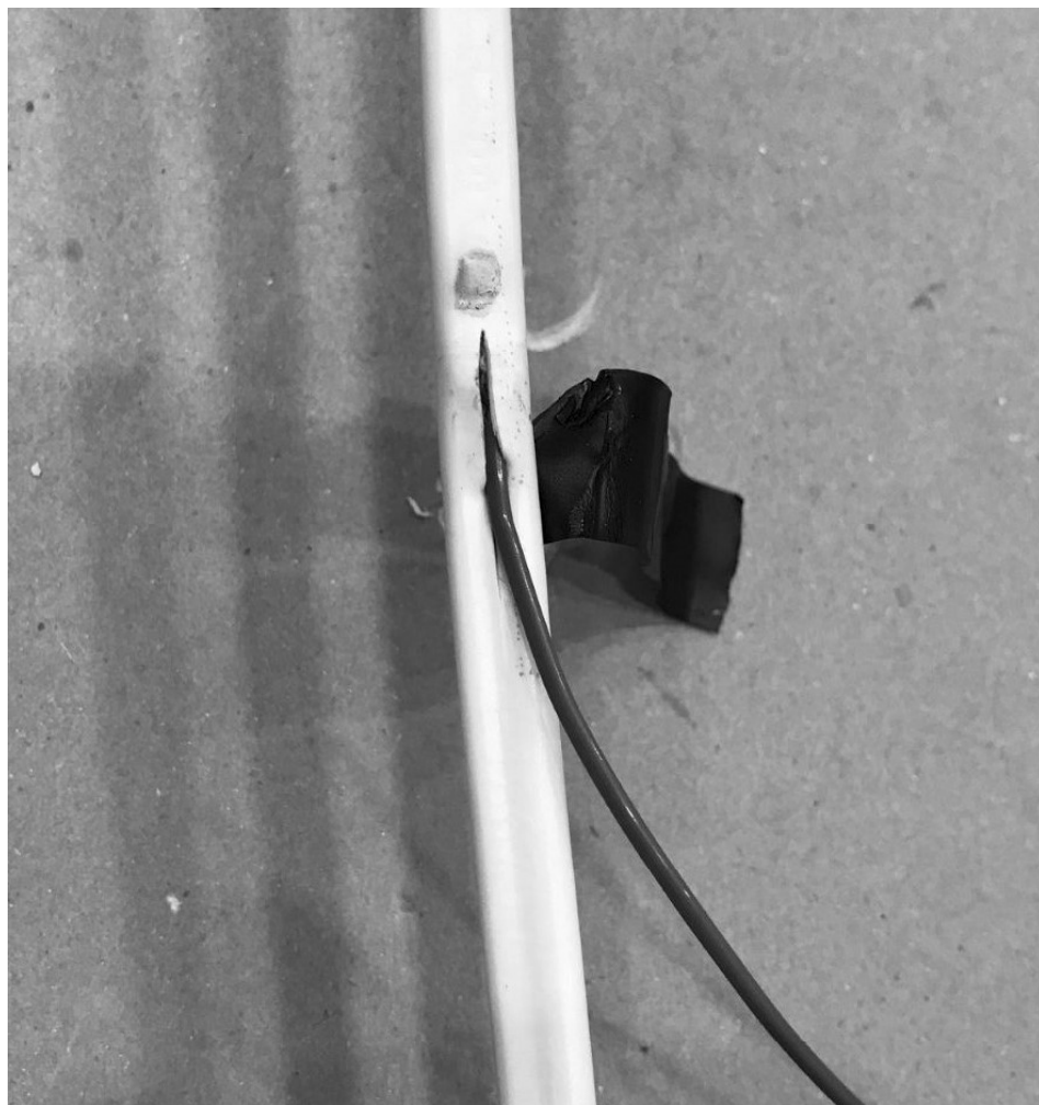
Figure B.2: Thermocouple Installed in NM-B Sample
