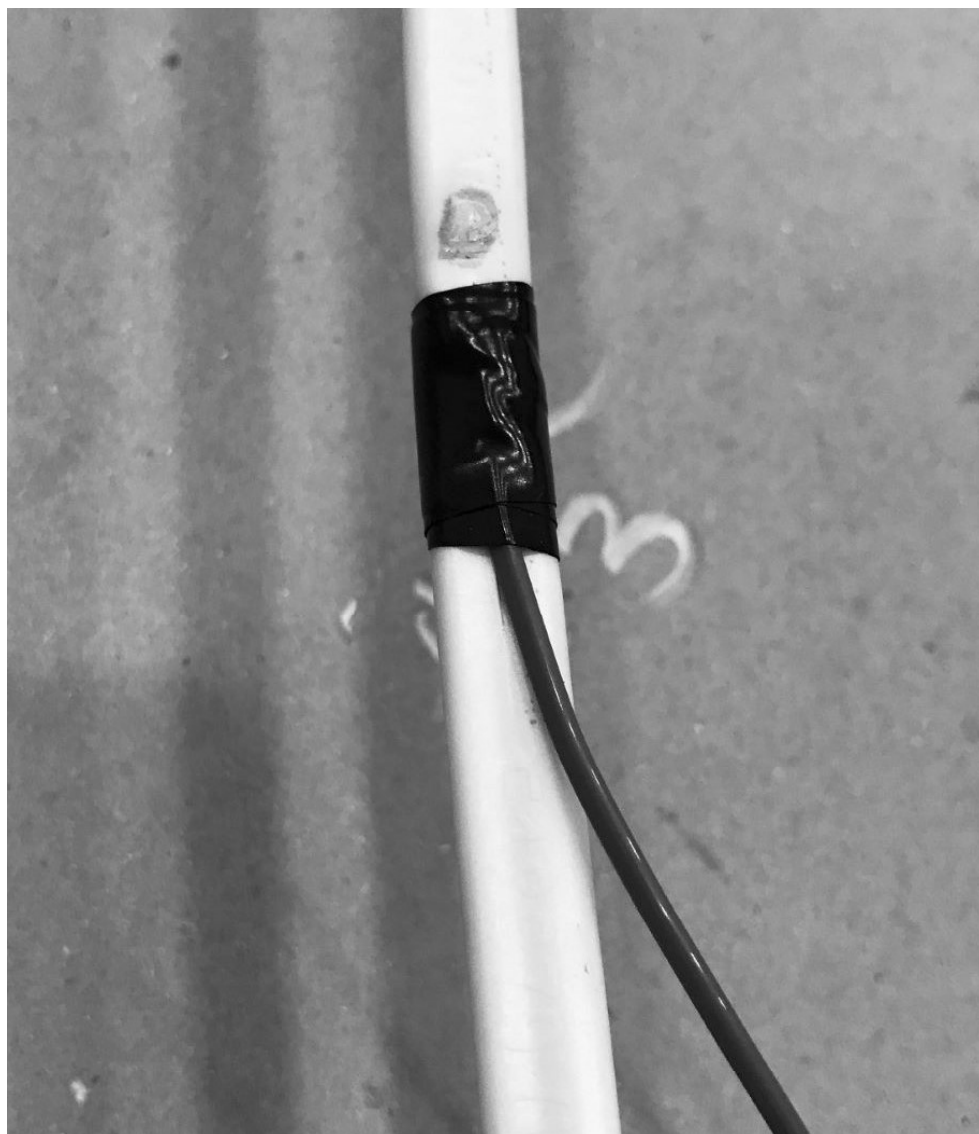
Figure B.3: Thermocouple Installed in NM-B Sample
