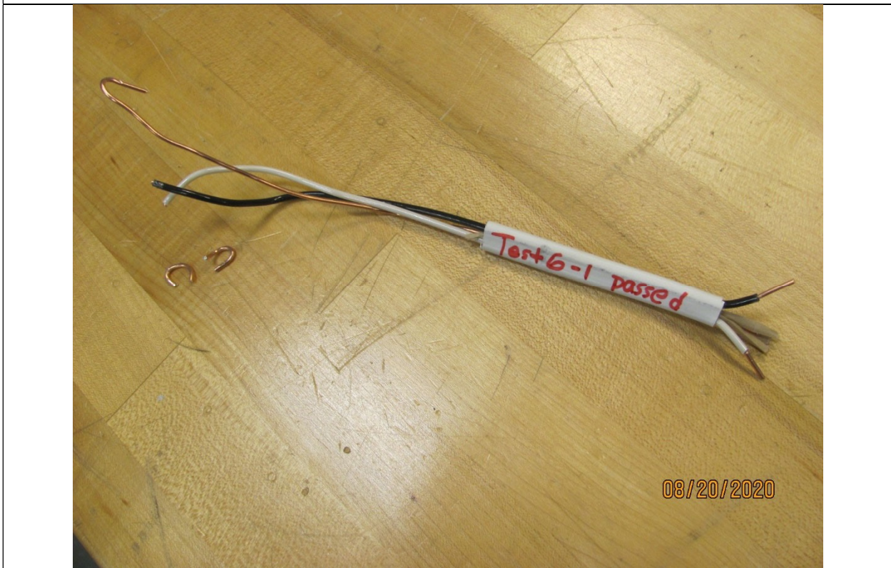
Photo 20 – Flexing Test Broken Conductors When Removing
