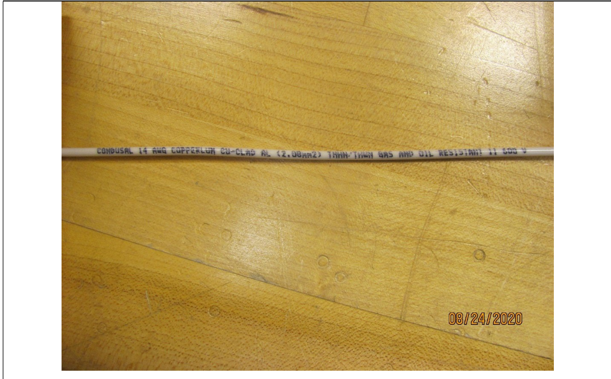
Photo 23 – Copper-Clad Aluminum THHN Sample Packaging at Eaton
