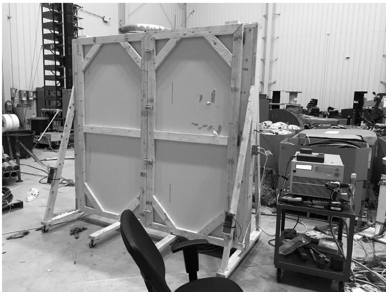
Figure B.5: Apparatus in Wall Configuration with Sheetrock Doors Closed
