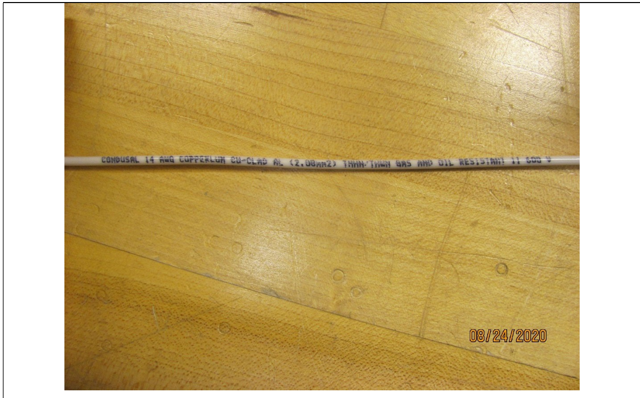
Photo 23 – Copper-Clad Aluminum THHN Sample Packaging at Eaton
