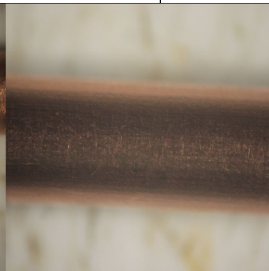
image 3: cohesion test (reverse torsion)
