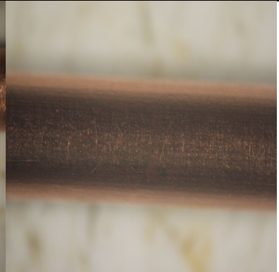
image 3: cohesion test (reverse torsion)
