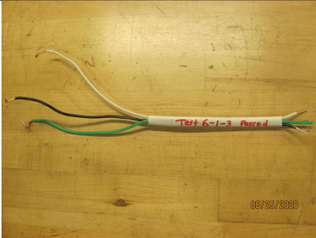
Photo 21 – Flexing Test Repeat No Conductor Breakage
