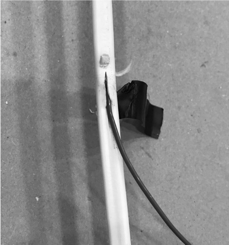
Figure B.2: Thermocouple Installed in NM-B Sample
