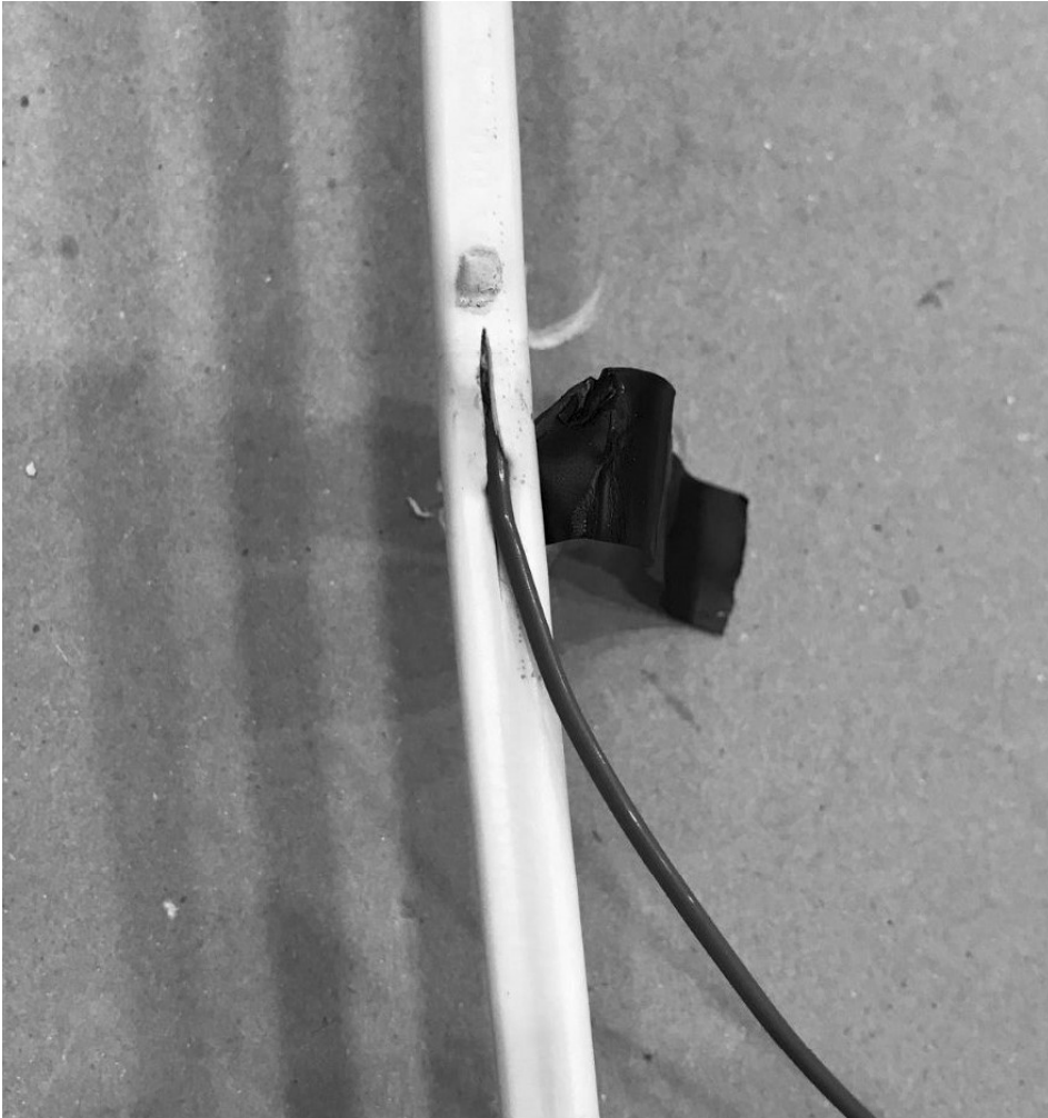
Figure B.2: Thermocouple Installed in NM-B Sample
