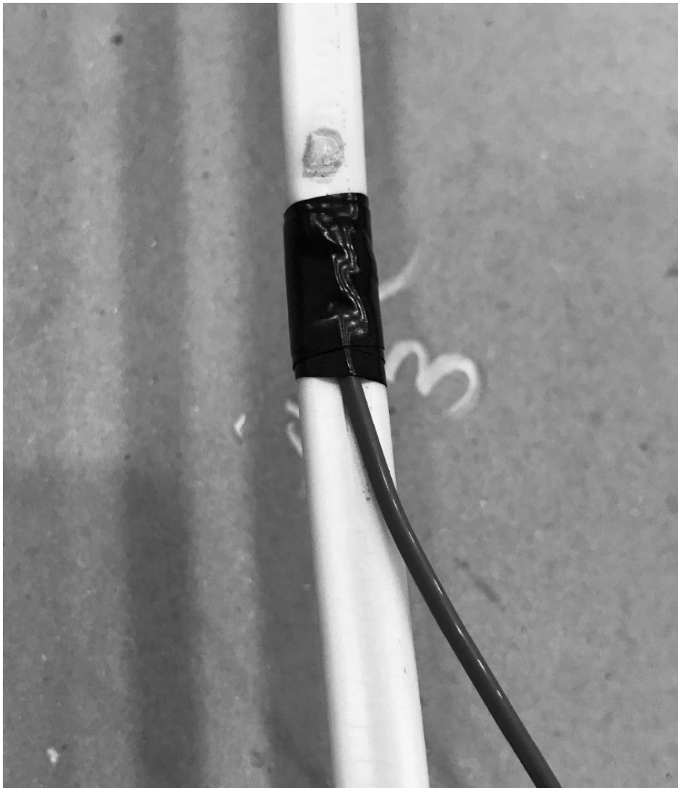
Figure B.3: Thermocouple Installed in NM-B Sample
