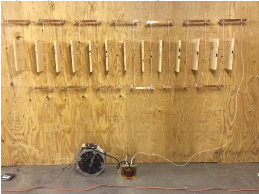
Complete Setup with 12 AWG Wire and Ideal, Wago, Gardner and Bender Connectors
