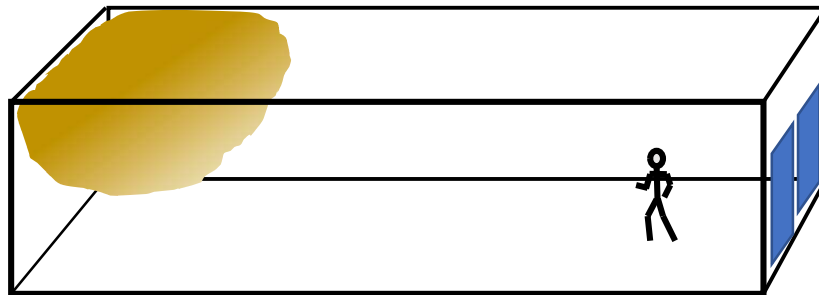
Figure AA.1: The Building Compartment Deflagration Scenario
