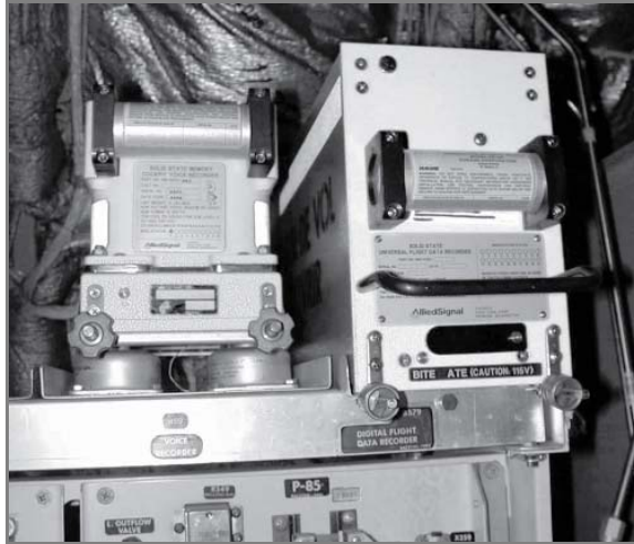
Figure 13.5(b) Location of Flight Data Recorder and Cockpit Voice Recorder.
