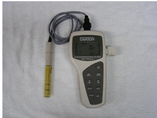
Figure A.6.2.2 (d) Conductivity meters are another device that can be used to measure the index of refraction. These devices are typically easy to use and have repeatable results. Following the user instructions of the device for calibration and cleaning requirements.
