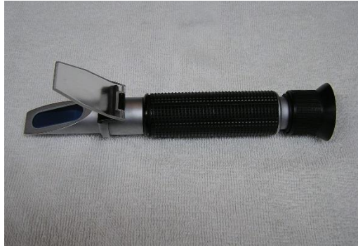
FIGURE A.6.2.2(a) Visual refractometer. Measuring the Index of Refraction by Placing a Few Drops of the Solution to Be Tested on the Prism of a Refractometer and Closing the Cover Plate. This is a typical refractometer suitable for this purpose. Holding this Type of Refractometer Up to a Light Source to Take a Reading Where the Dark Field Intersects the Numbered Scale.
