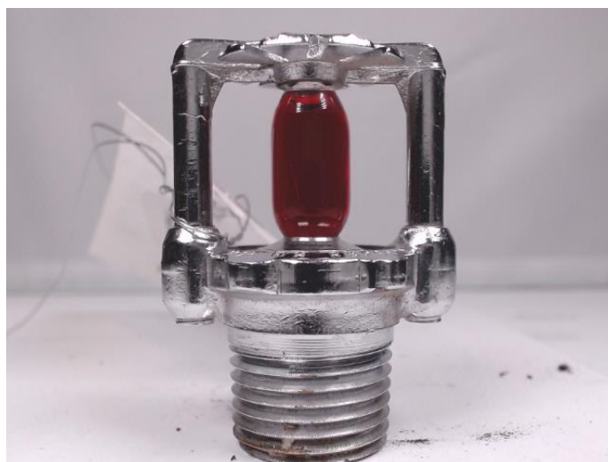
Figure 6. Older Standard Response Sprinkler Used
