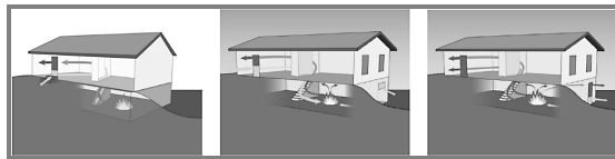
Figure 12.7.1.1 Diagrams Representing Exterior No-Access Basement (left), Limited-Access Basement (middle), and Full-Access Basement (right). (Courtesy of UL Fire Safety Research Institute.)
