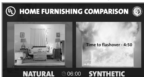
Figure 4.6.1 Synthetic Fuel and Natural Fuel Fire Comparison.
