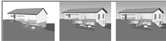
Figure 12.19.1 Diagrams Representing Exterior No-Access Basement (left), Limited-Access Basement (middle), and Full-Access Basement (right). (Courtesy of UL Fire Safety Research Institute.)
