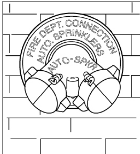
Figure 4.2.1 Fire Department Connection to Automatic Sprinkler Systems.
