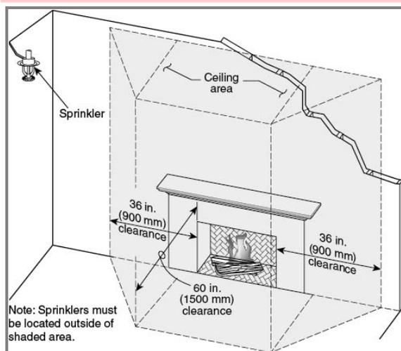
**Figure A.7.5.6.3(3)(b) Open Fireplace Recessed Fireplace — Intermediate Temperature Sprinkler Location .**
