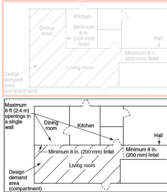
**Figure A.10.2(b) Sprinkler Design Areas for Typical Residential Occupancy — Without Lintel Between Dining Room, With Lintel Between Hall .**
