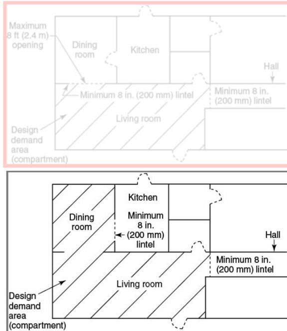
**Figure A.10.2(c) Sprinkler Design Areas for Typical Residential Occupancy — Without Lintel Between Adjoining Spaces: Dining Room and Hall.**
