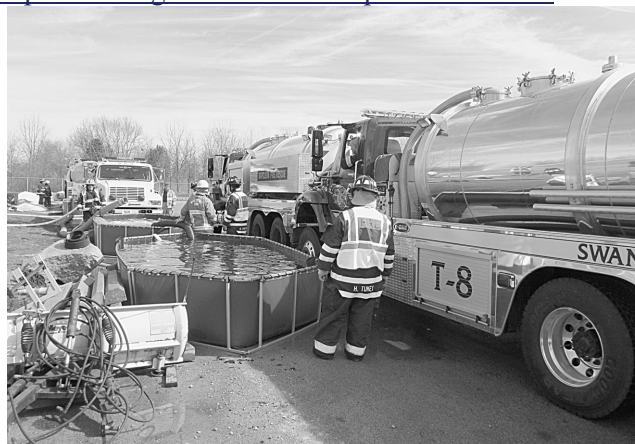
Figure C.5.2.3.2.1 Folding Frame Tanks with Narrow Profile Configuration Deployed In-Line with a Supporting Pumper Leaving a Travel Lane Open for MWSA.
