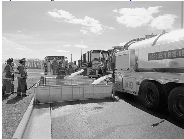
Figure C.2.4.2.6.2 Dump Site Configured to Simultaneously Service Two MWSA ( Kd = 2 ).
