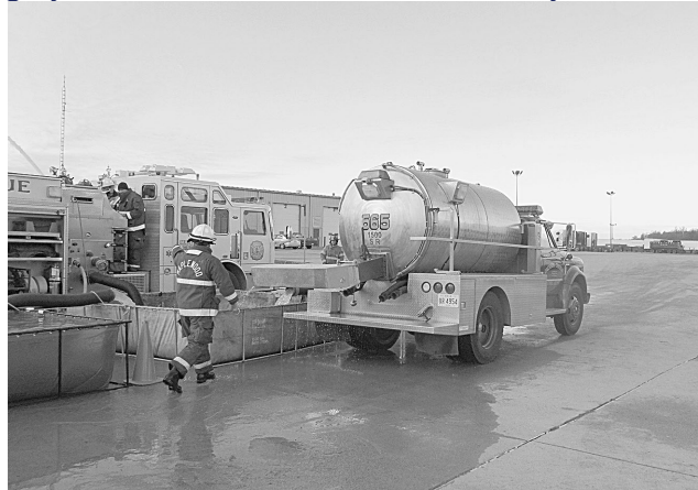
Figure C.2.2.2.2.1 Legacy MWSA with Circular Tank Geometry, Converted from Civilian Use.
