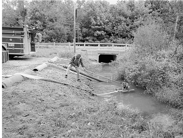
Figure C.3.3.4 Floating Portable Pump Used in Support of Fill Site Operations During a Water Shuttle.
