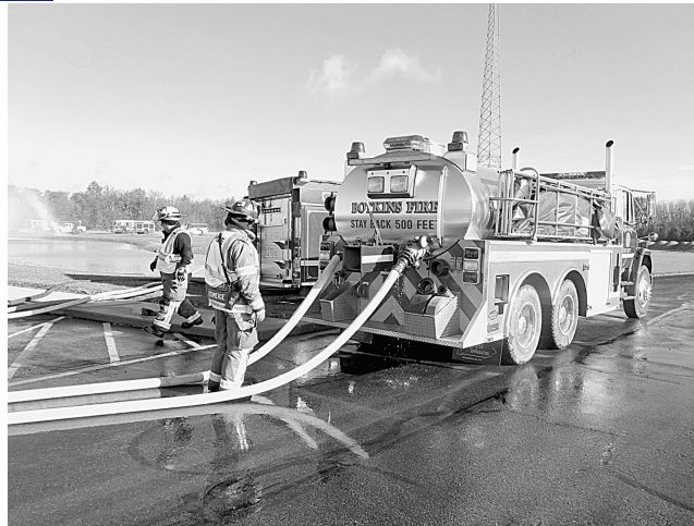
Figure C.2.2.3 Typical Arrangement of Dual 2 1/2 in. (65 mm) Fill Connections Located on the Rear of an MWSA Tank.
