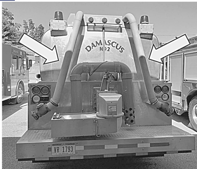
Figure C.2.2.3.1 Fill Port Pipe Extensions Retrofitted to an Older Apparatus to Allow Safe Access by Ground Crew.
