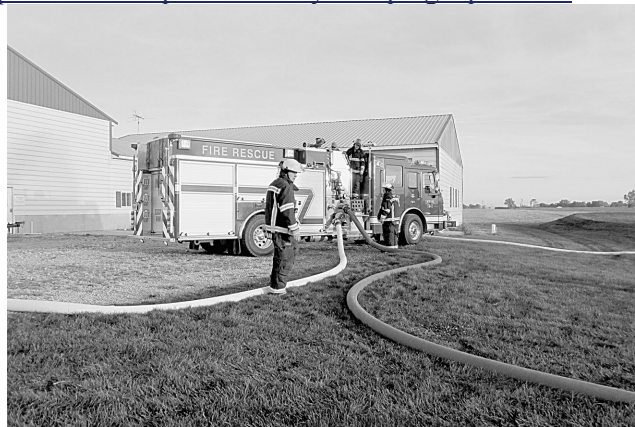
Figure C.3.2 Fire Department Pumper in a Relay Pumping Operation.
