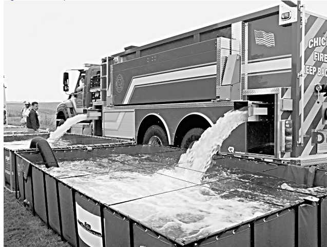
Figure C.2.2.4.2.1 Large Capacity MWSA [4000 gal (15,000 L)] Equipped with Multiple Transfer Outlets (Dump Chutes) to Decrease Offload Time.
