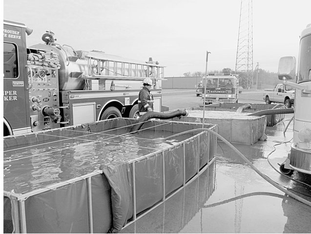
Figure C.5.3.1 Water Transfer Using Jet Siphons from Dump Tanks to Draft Tank (Center) at a Water Shuttle Dump Site.
