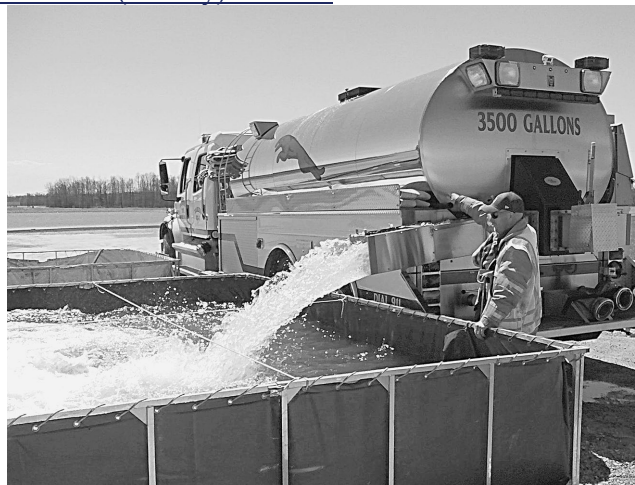
Figure C.2.2.1.1 Conventional (Gravity) MWSA.
