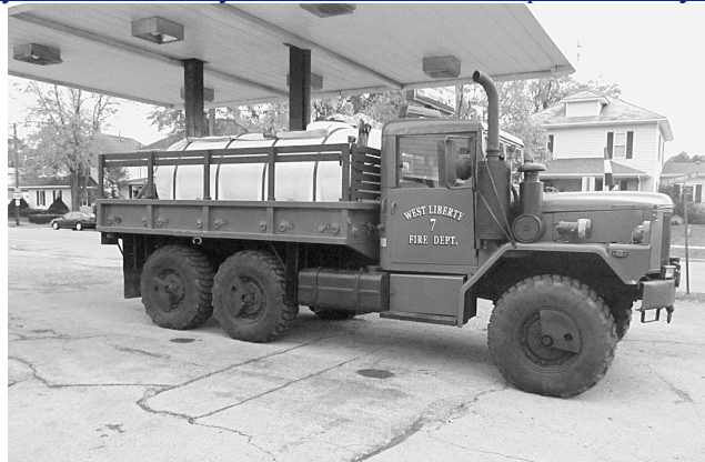
Figure C.2.5.1 Legacy MWSA Locally Converted from a Surplus Military Truck.
