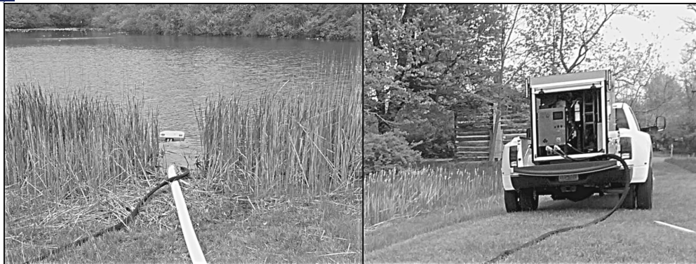
Figure C.3.3.4.1 FSSP Deployed in Static Source (Left) and Shore-Based Hydraulic Power Unit (Right).
