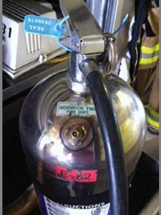
Modified extinguisher shell with added Schrader valve.
