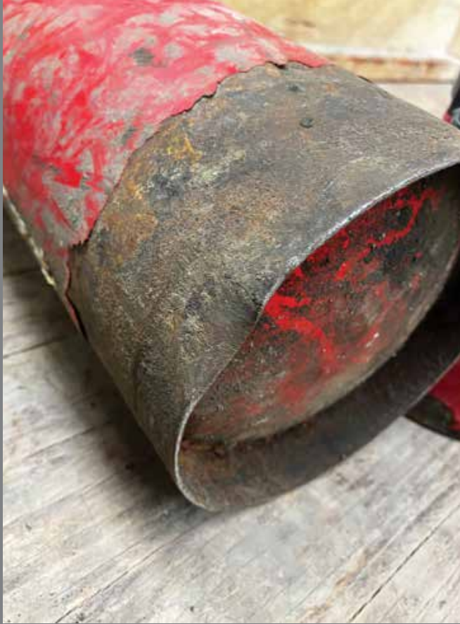
Damaged extinguisher: dented skirt, corroded shell, peeled paint.
