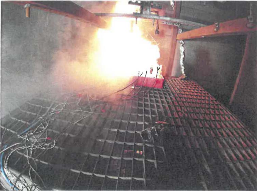
Figure 2: View into the test chamber after inducing a thermal runaway by ignition of the two glow plugs. Above the battery package the two nozzles for introduction of the extinguishing agent (water and 2% F500) are shown.
