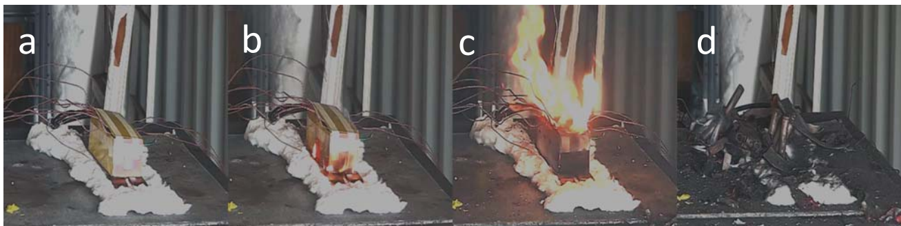
Fig. 2 Four sequences of free burn of a 12 V battery pack fire ( a smoke starts, b flame starts, c explosion, d burnout)
